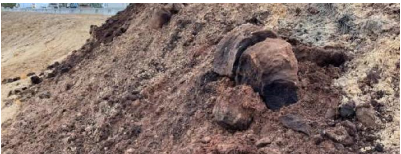
Figure 17 Coffee rocks and cinders stockpiled before liming treatment
