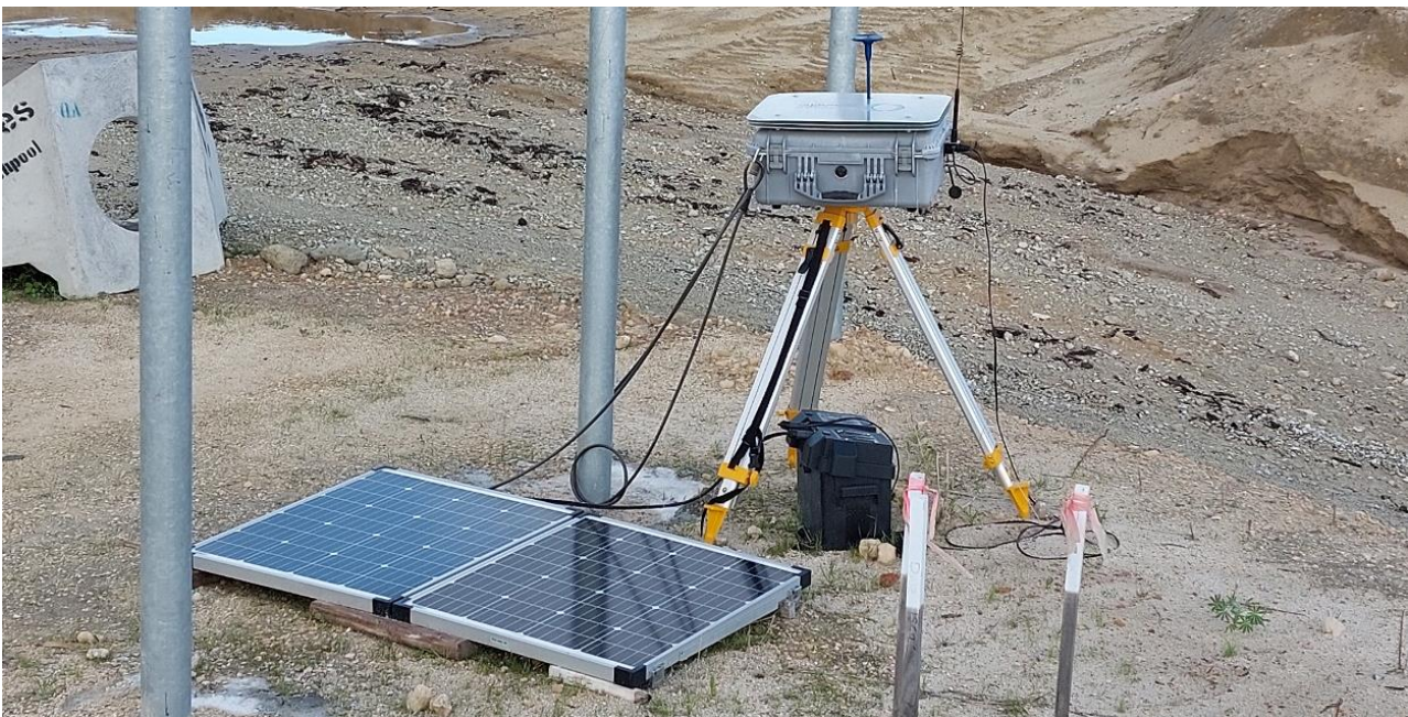
Figure 15 DustTrak on the eastern side of southern dive structure
